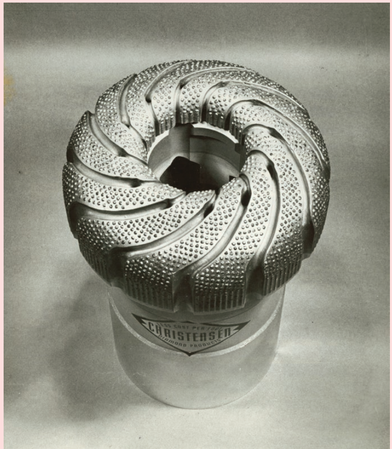
About 2,500 diamond stones pave the surface of a core drill crown produced for Project Mohole. Image courtesy National Academies Archives
