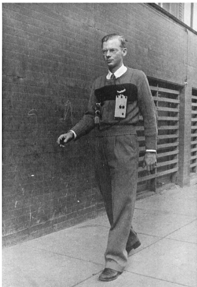
Holter's original wearable health technology: the radioelectrocardiograph, c. 1957. Courtesy of the New York Academy of Sciences.
